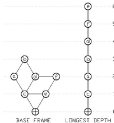
Figure 6 - J-graphs for the base frame (left) and its theoretical longest configuration (right)
