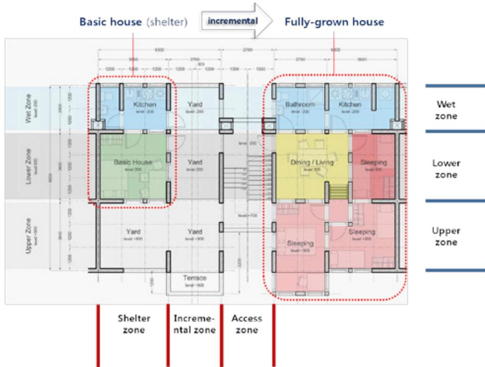
Figure 5 - The Basic House and the Fully grown House (copyright: Kyung W Seo, 2016)
