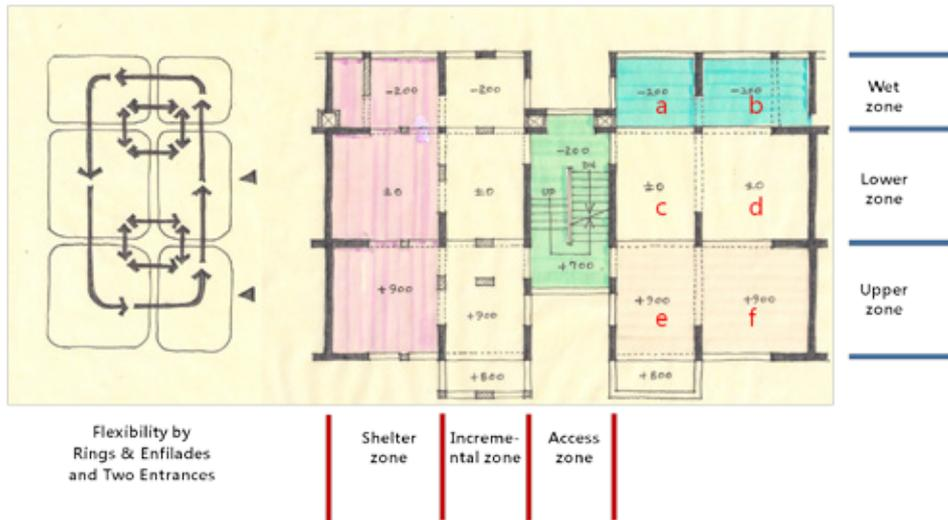
Figure 3 - Concept and Zoning of Incremental Housing (copyright: Kyung W Seo, 2016)
