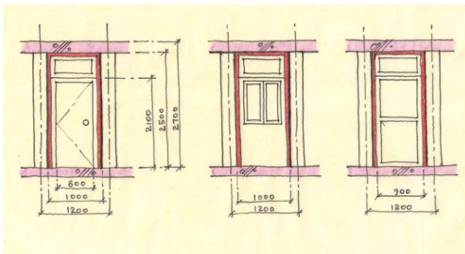
Figure 4 - Three basic components with the same module (copyright: Kyung W Seo, 2016)
